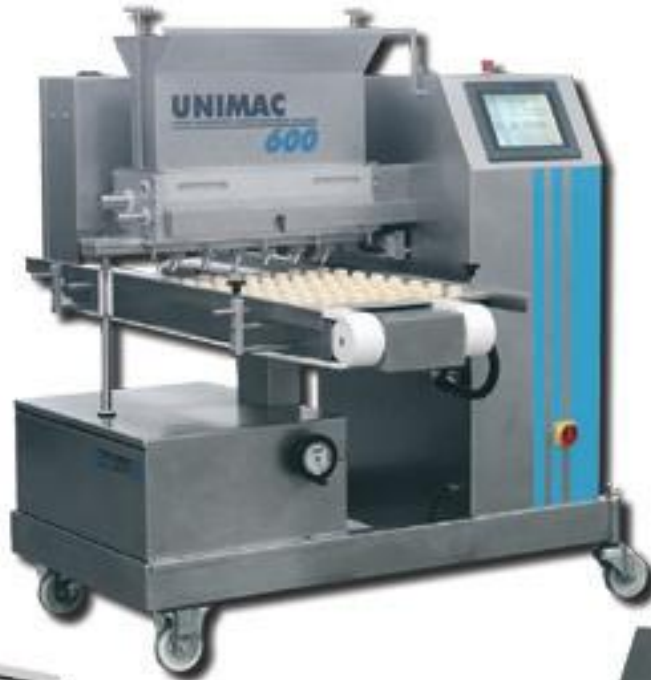
3-roll extruding head Designed for heavy doughs and masses like cookie dough, cocos, spritz etc.
